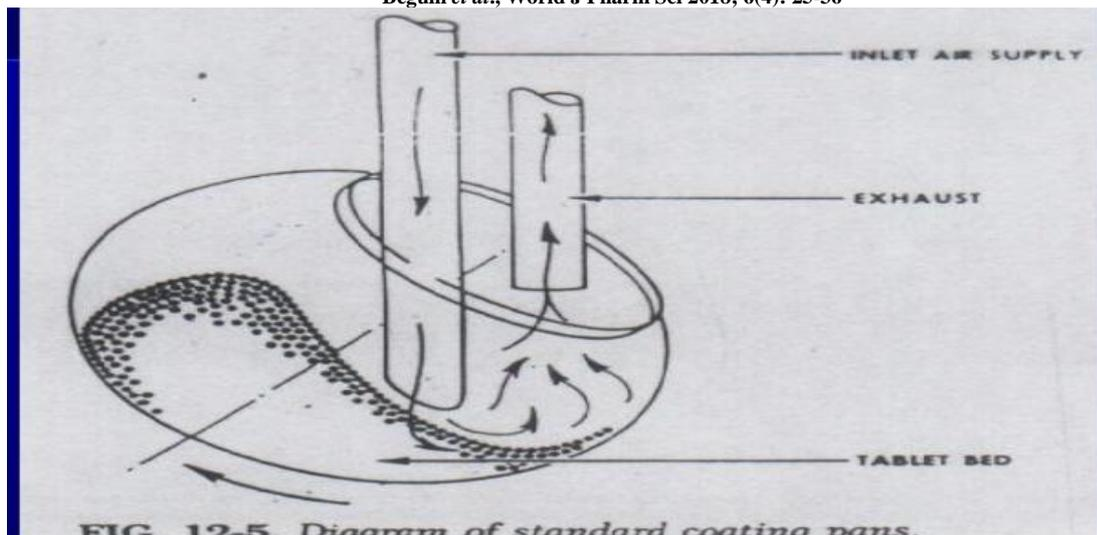
FIG. 12-5. Diagram of standard coating pans.
